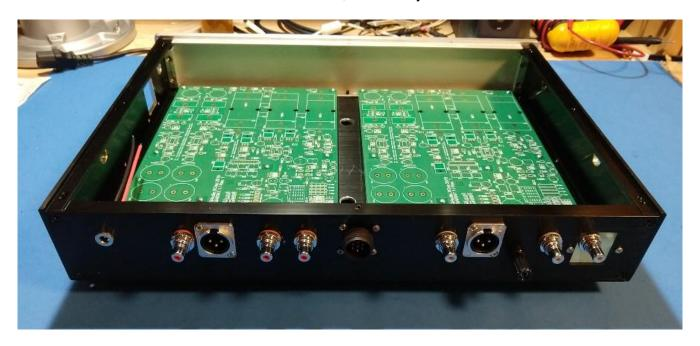
Had to fill the power connector hole for the RCA. The RCA connectors shown were not the final ones installed.
