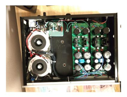
MuMetal over power section is shown below. MuMetal is under the transformers and on the sides as well. Another is on the case top.
