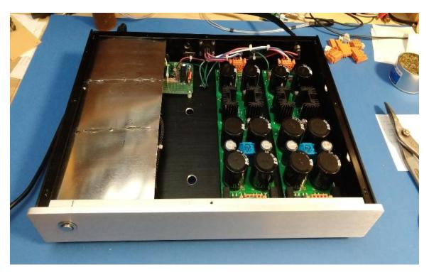
XONO preamp case: Notice the lack of coupling capacitors near the front panel
